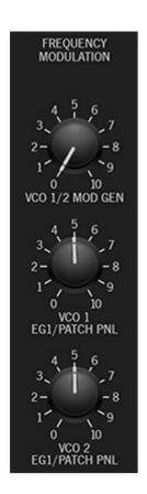
Don't forget to turn up the *VCO 1* and *VCO 2 EG1/Patch Panel* attenuators in the Frequency Modulation section - these regulate the amount of signal received through the VCO *Freq* mod jacks.
