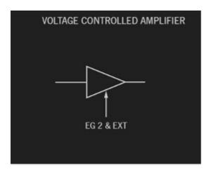
Outside of a modulation attenuator, PS-20's main VCA doesn't any controls, per se, but it's helpful to understand its functionality.
