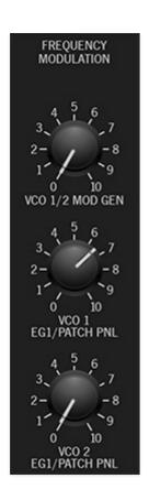
You'll need to turn up the *VCO 1 EG1/Patch Panel* attenuator in the Frequency Modulation section to hear the Sample & Hold modulation.
