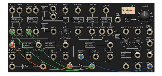
The Modulation Generator saw/triangle/ramp output is patched to the auxiliary VCA *In* (orange cable), and the auxiliary VCA *Out* is multed to both VCO 1 and VCO 2's *Freq* mod inputs. The Mo*d Wheel* output jack is then patched to the auxiliary VCA *Control* input (blue cable). In this way, the mod wheel regulates the signal flowing through the VCA, i.e. the amount of signal traveling from the mod generator to the oscillator frequency mod inputs.
