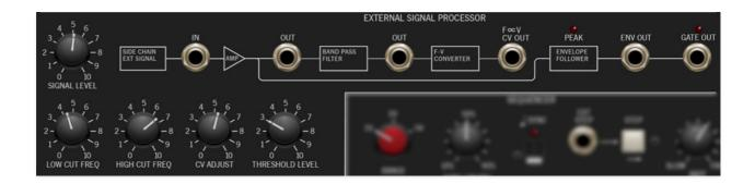
PS-20 includes a full recreation of the slightly bizarre and endlessly useful External Signal Processor section of the classic MS-20 synthesizer.
